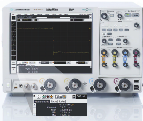
The 32-GHz members of the Infiniium 90000 X-Series exhibit 10 to 90% rise and fall times of just 13 psec and little noise or jitter.
