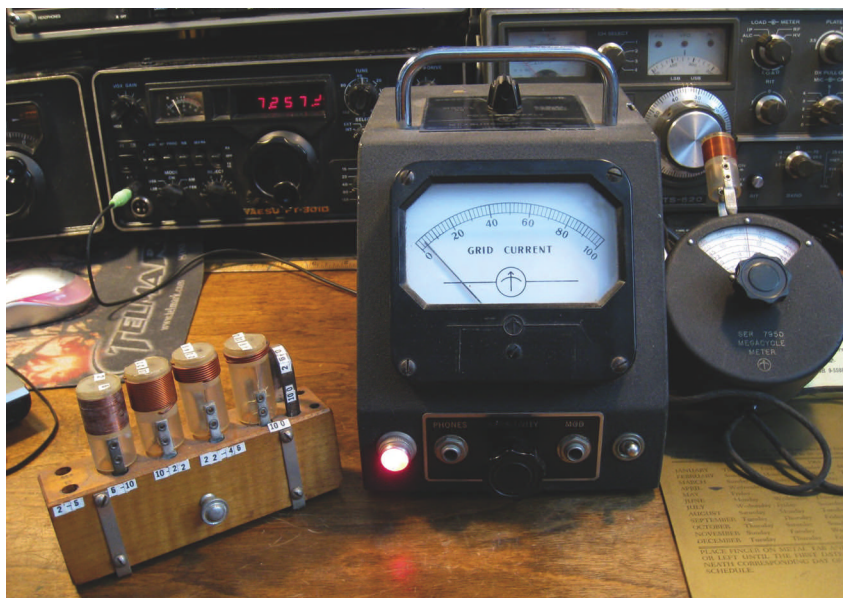
Figure 1 If you have the experience, you can design your RF circuits with a Boonton Measurements Corp Model 59 Grid-Dip meter, sold in 1947, in lieu of more expensive test equipment (courtesy Ken Blume, K2UPI).
